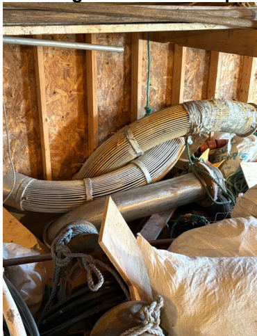
dewatering elbows for fish pump
